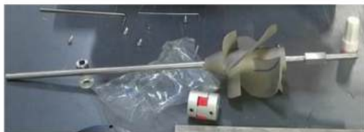
Fig. 4 Components of impeller and drive train assembly
