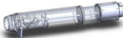
Fig. 1 3D CAD rendering of waterjet propulsion system
