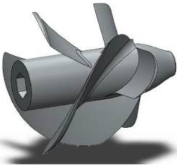
Fig. 5 CAD rendering of 4-blade twisted impeller
